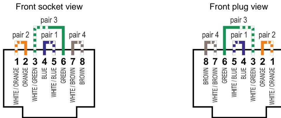
Obr. 3 - Socket and plug wiring
