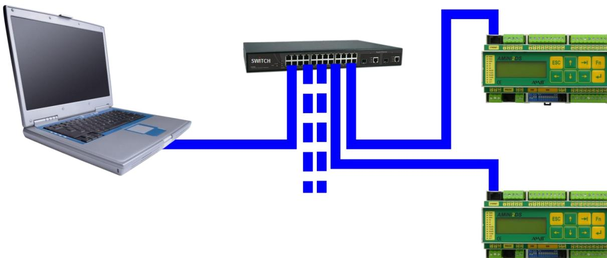
Obr. 2 - Connection of multiply units to the network
