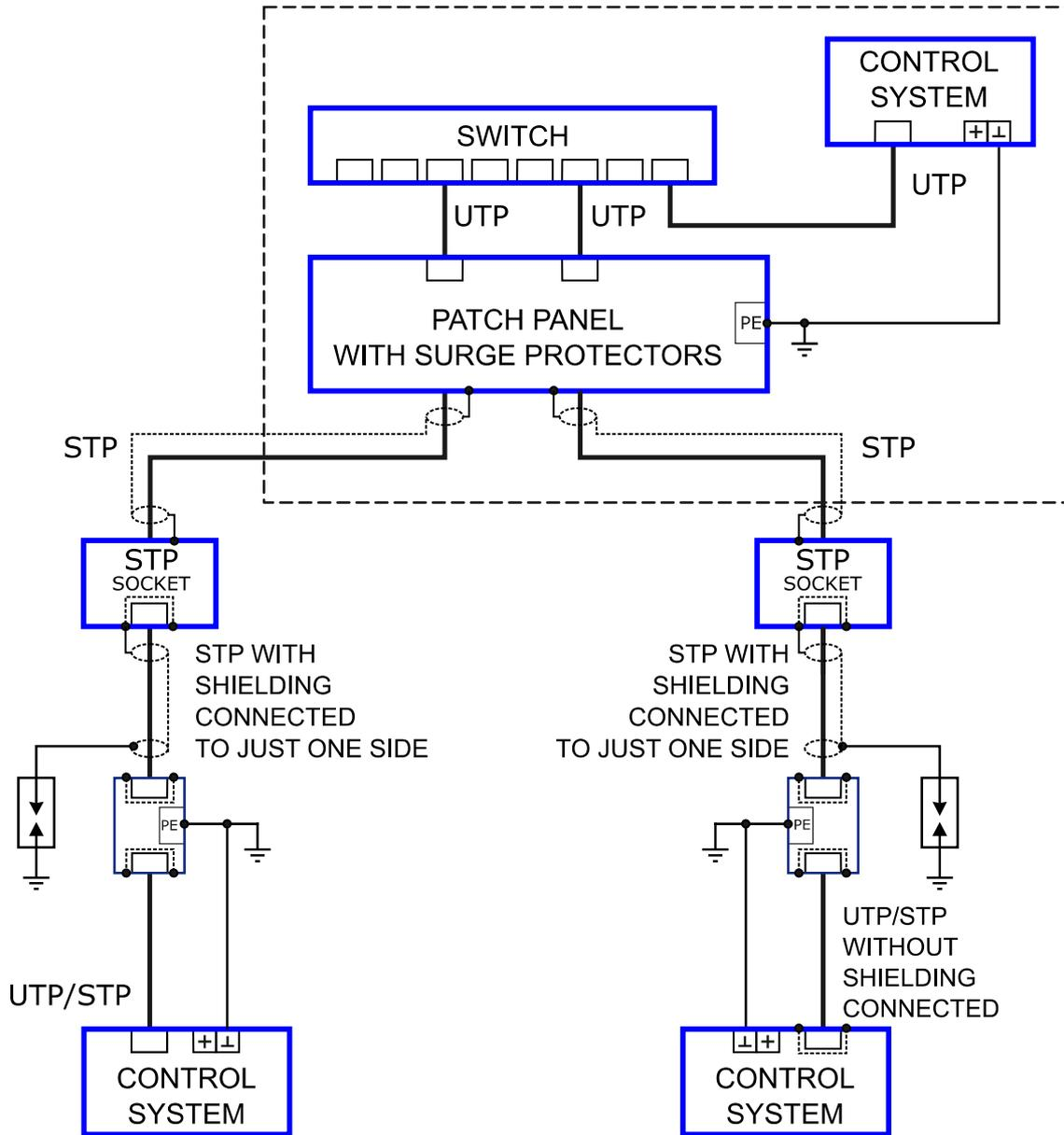
Obr. 5 - Surge protection wiring in network Ethernet
