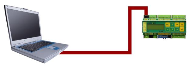
Obr. 1 - Direct PC connection with control system
