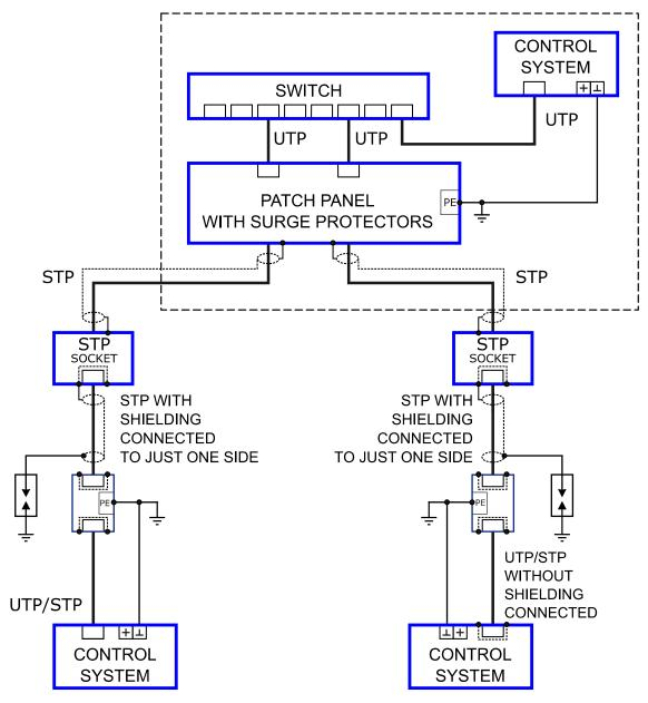
Obr. 5 - Surge protection wiring in network Ethernet
