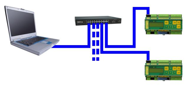
Obr. 2 - Connection of multiply units to the network
