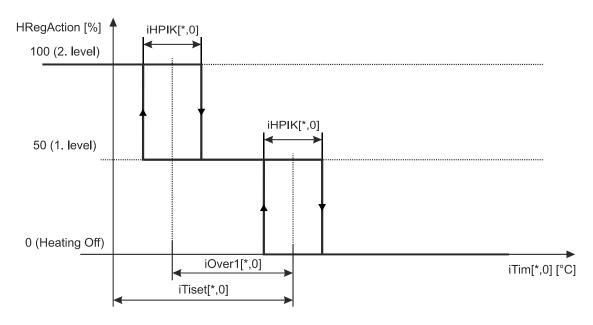
Fig. 7 – Two-level heating control
