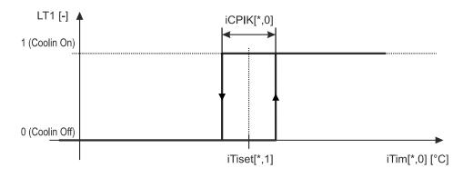
Fig. 6 – ON-OFF cooling control
