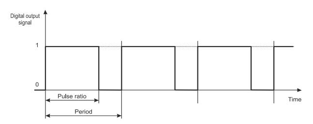
Fig. 4 – Pulse width modulation
