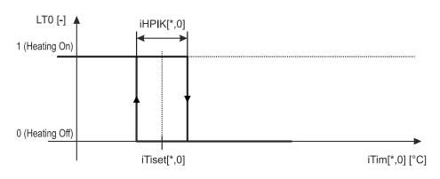
Fig. 5 – ON-OFF heating control
