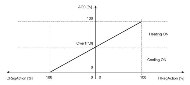
Fig. 9 – Conversion of action variables to the analogue output of the sequence control
