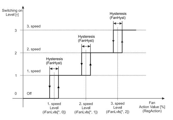
Fig. 3 – Automatic control of a three-speed fan
