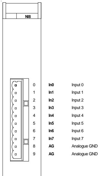
Note: The AG terminals are internally connected with  $\perp$  (the GND terminal) at the AD-CPU167 power supply connector.
