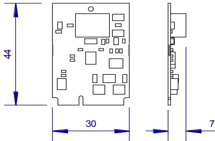
The **EM-CAN** module is to be connected exclusively to compatible products manufactured by the AMiT company. Connecting it to a different device utilising the miniPCIe slot may result in damage both to the device and to the connected **EM-CAN** module. The manufacturer not bear any responsibility for damage caused this way. Failure to observe this also voids the warranty. Communication module installation instructions can be found in the operation manual of the respective compatible device.
